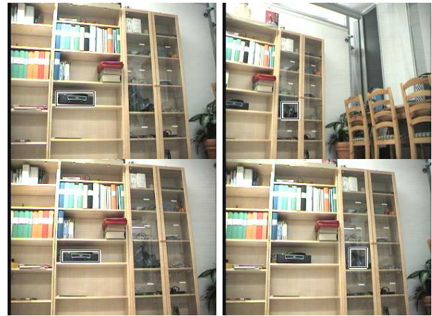
Fig. 8. The rectangles denote correctly matched ROIs. Top: current frame. Bottom: frame with expected ROI from database. Left: “easy” matching situation. Right: “difficult” matching situation from different viewpoint.
