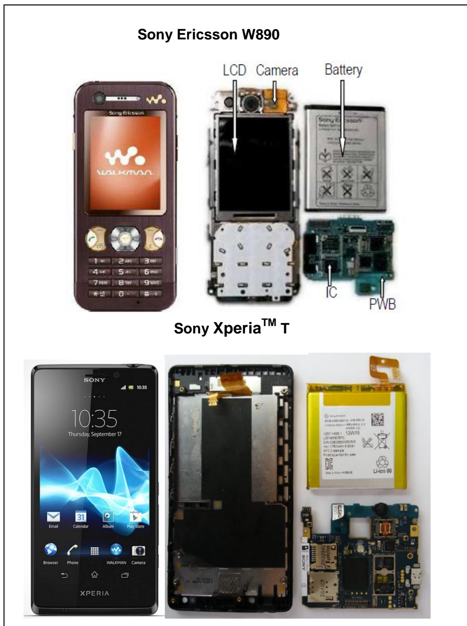
Figure 2 Image of feature phone, Sony Ericsson W890, used in the previous, 2008 LCA study and the Sony Xperia™ T used in this study.
