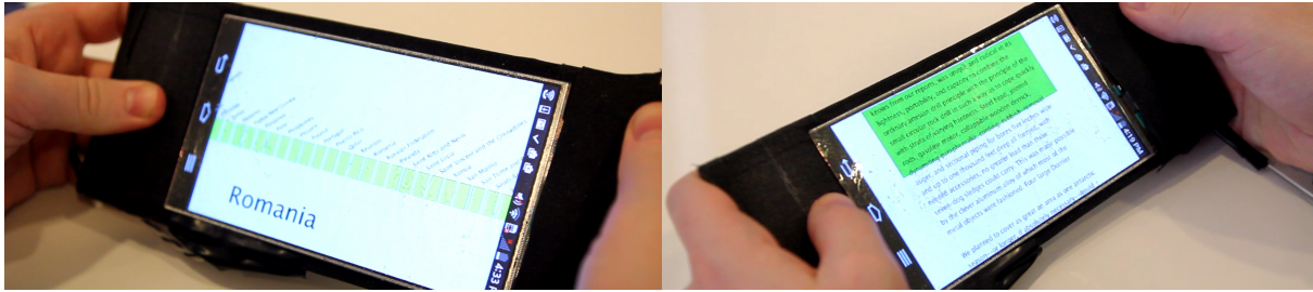
Figure 3. Left: Using A-RC for off-screen browsing of large lists, and combination R-PC for selecting on-screen items in the list. Right: Using R-PC for scrolling a text, and A-RC for annotating items.
