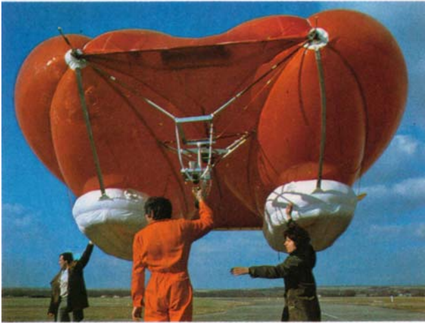
Fig. 15. French double trilobed airship 'Dinosaure'
