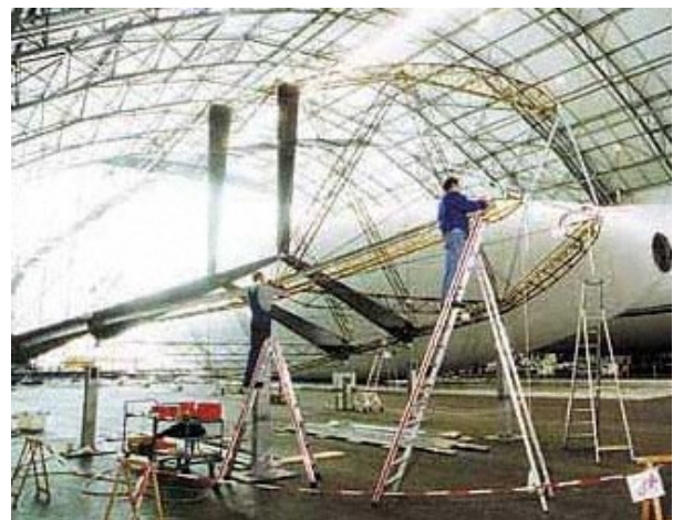
Fig. 22. Triangular frames and longerons in Zeppelin NT
