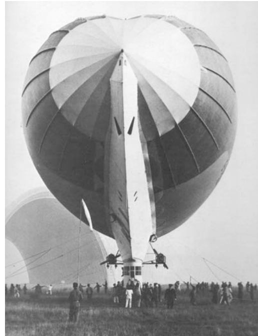
Fig. 21. French Zodiac bi-lobed airship "E-8"
