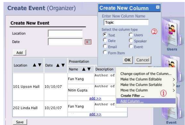
Figure 6: Adding the topic column to the presentation nested table. The resulting table is shown in Figure 2.
