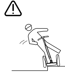
Figure 36: Do Not Drop a Wheel off a Curb
