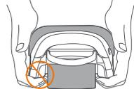
**!** Do not lift the Segway Drift when powering on or after powered on. The wheels will spin, causing a high risk of injury.
