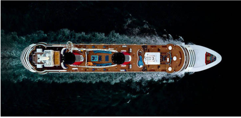
Disney Dream from above, showing the private sun deck above the bridge, Mickey's Pool, the two funnels amidships [the forward funnel is a dummy], and Goofy's Sports Deck athwartships and aft. Jeffrey Milstein, "Disney Dream 02," archival inkjet on paper. Courtesy Foster/White Gallery.
