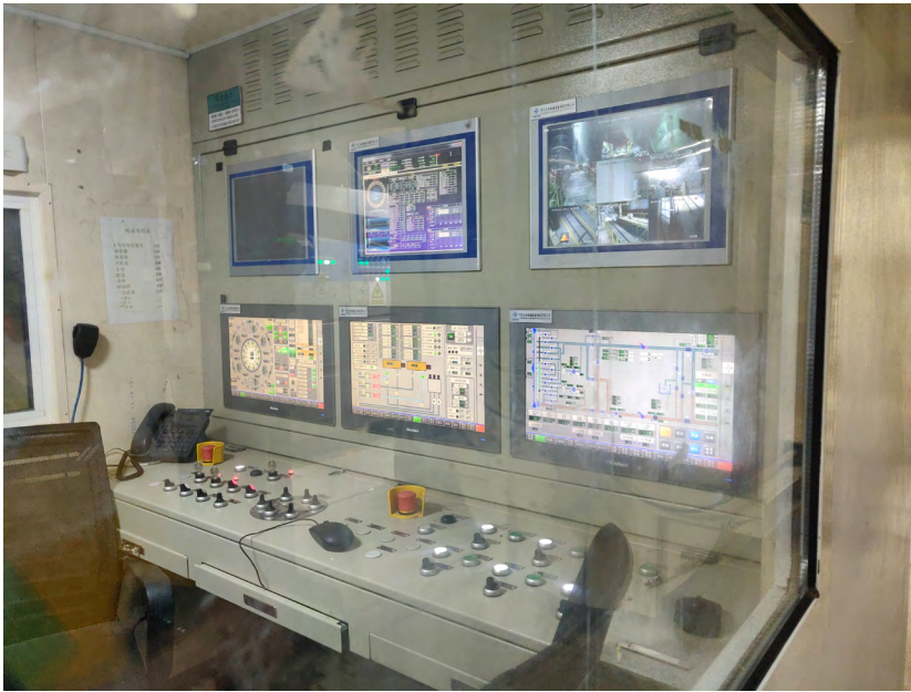
Tunnel-boring machine control room, taken underground inside the tunnel space of the boring machine. Courtesy of the author.
