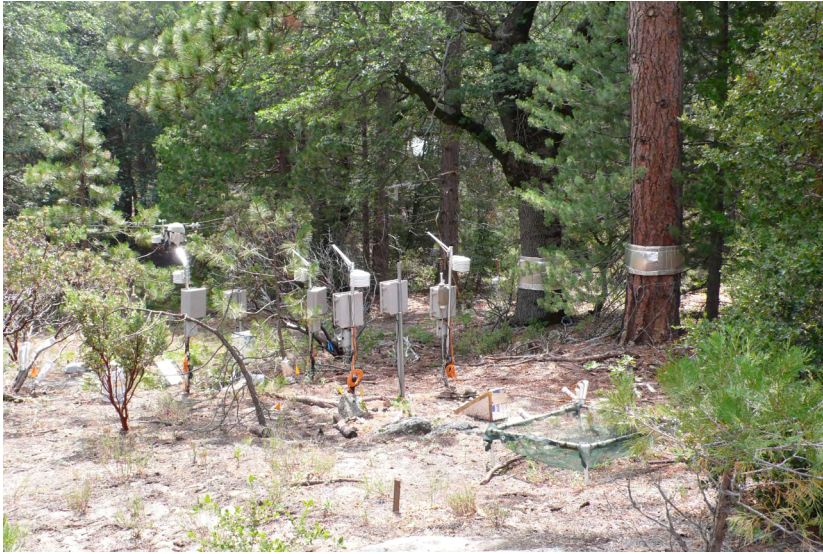
An array of sensors at James Reserve measuring moisture and respiration of CO 2 throughout the soil. Photograph by Jennifer Gabrys, 2008.
