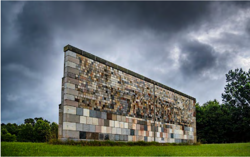
The stone test wall at the NIST headquarters in Gaithersburg, MD. Reprinted with permission from the National Institute of Standards and Technology [2018, rights reserved]. Photograph by Jason Stoughton.
