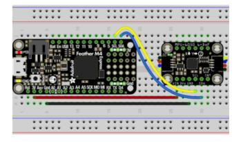
Board 3V to sensor VIN (red wire)
