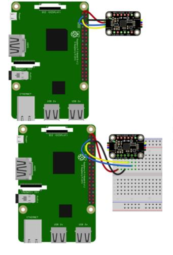
Pi 3V to sensor VCC (red wire)
