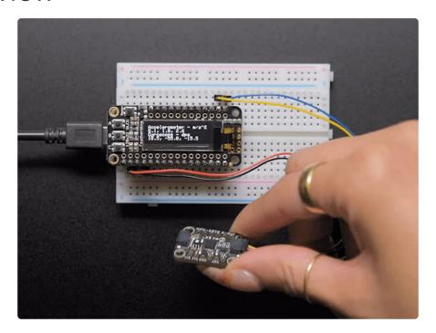
The MPU-6050 is a popular six DoF accelerometer and gyroscope (gyro) that has all the info you need on how things are shakin' and spinnin'. With six axes of sensing and 16-bit measurements, you'll have everything you need to give your robot friend a sense of balance, using the MPU-6050 as its inner ear.
