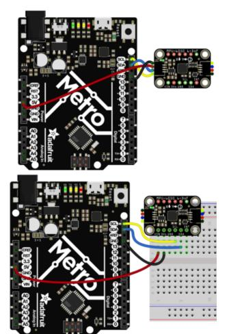
**5V** if you are running a **5V** board Arduino (Uno, etc.). If your board is **3V**, connect to that instead.
