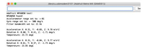
Give the sensor a wiggle or a spin and watch how the measurements change!
