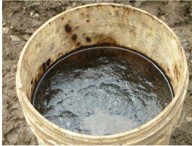
Figure II-4 Oil floating on the top of water purged from a monitoring well adjacent to Pit 3.
