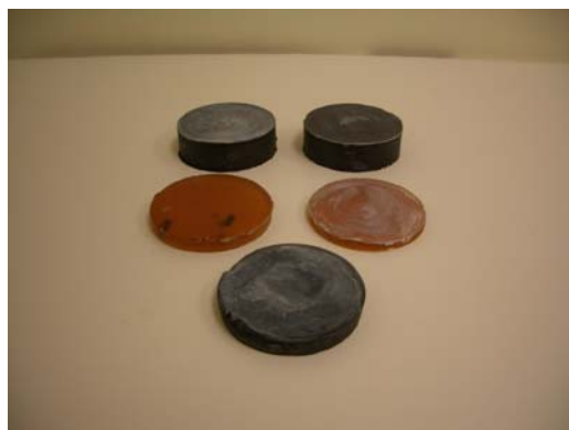
Figure 4.2 Samples of Derakane 8084 vinyl ester resin with or without additives
