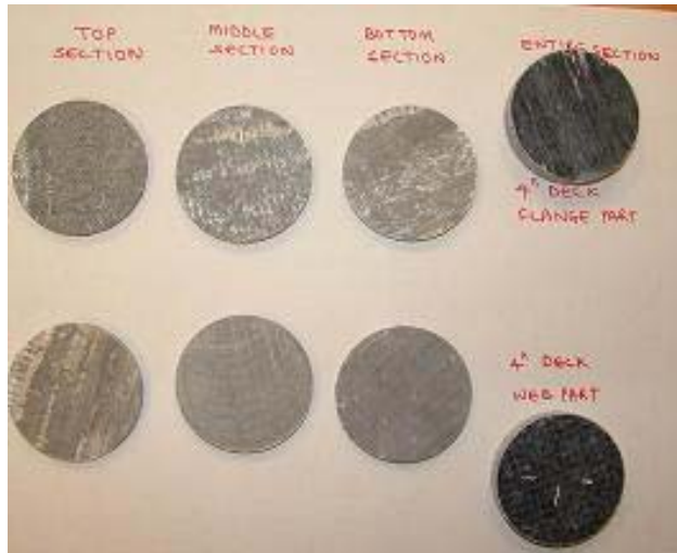
Figure 4.8 Samples prepared from web and flange sections of Prodeck 4
