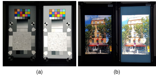
Figure 1. Picture (a) shows the proposed setup for measuring the capacity of MI devices to capture HDR scenes. The target contains a color chart, a texture chart, and a grayscale of 80 uniform patches linearly distributed between 0 and 100% of transmittance. The luminance of the left light source is always 170 \text{ cd/m}^2 . The luminance of the right light source varies between 170 and 17000 \text{ cd/m}^2 . In (b) a real scene is displayed in order to correlate the measurement with a perceptual analysis.
