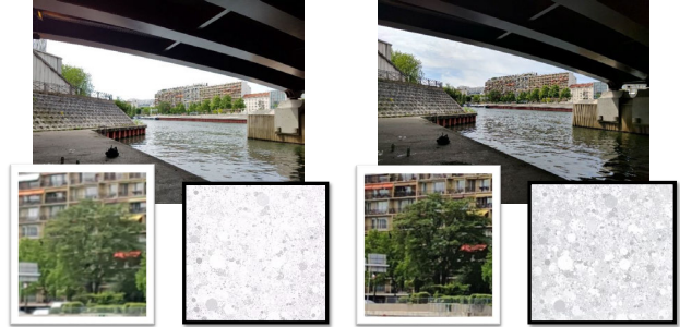
Figure 3. Comparison of quality attributes observed in natural and laboratory setups. The two photos correspond to different devices observing the same natural scene under the same conditions. The proposed objective measurements are scene independent and allow to study the rendition by the same devices in a controlled laboratory setting. For instance, the textures shown in the bottom-right (called Dead Leaves pattern) are used in the laboratory to evaluate the texture preservation. Note that in the laboratory shots, textures are reproduced similarly to the textures captured in the natural setting (crops in the bottom-left).
