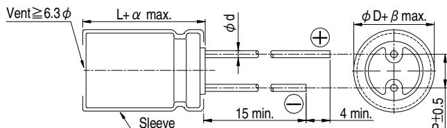
Lead Spacing and Diameter Unit: mm
