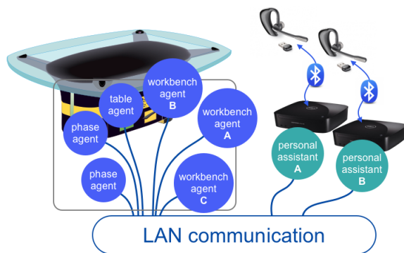
Figure 3: Simplified TATIN-PIC architecture showing the connection between the JADE Java agents (left) and the OMAS Lisp agents (right)
