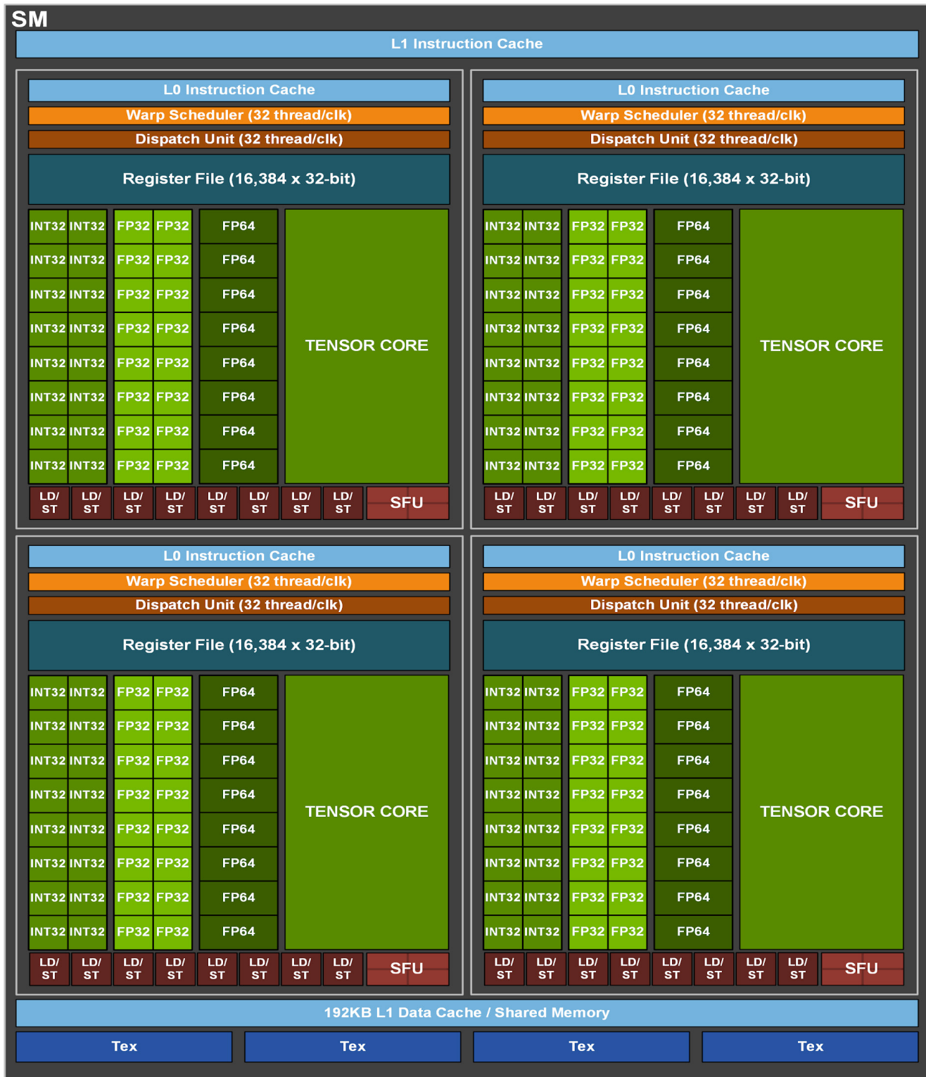
Figure 7. GA100 Streaming Multiprocessor (SM)
