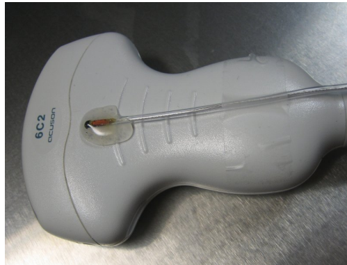
Figure 5.9.: Magnetic tracking sensor hot-glued onto the ultrasound probe.
