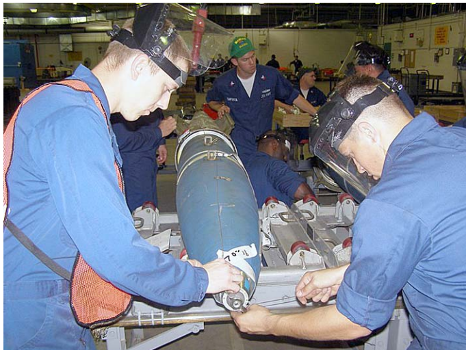
MN1 Joseph Pawlikowski instructs MN3 Gilbert Priest on the proper routing of the arming wires on a MK63 Quick Strike.
