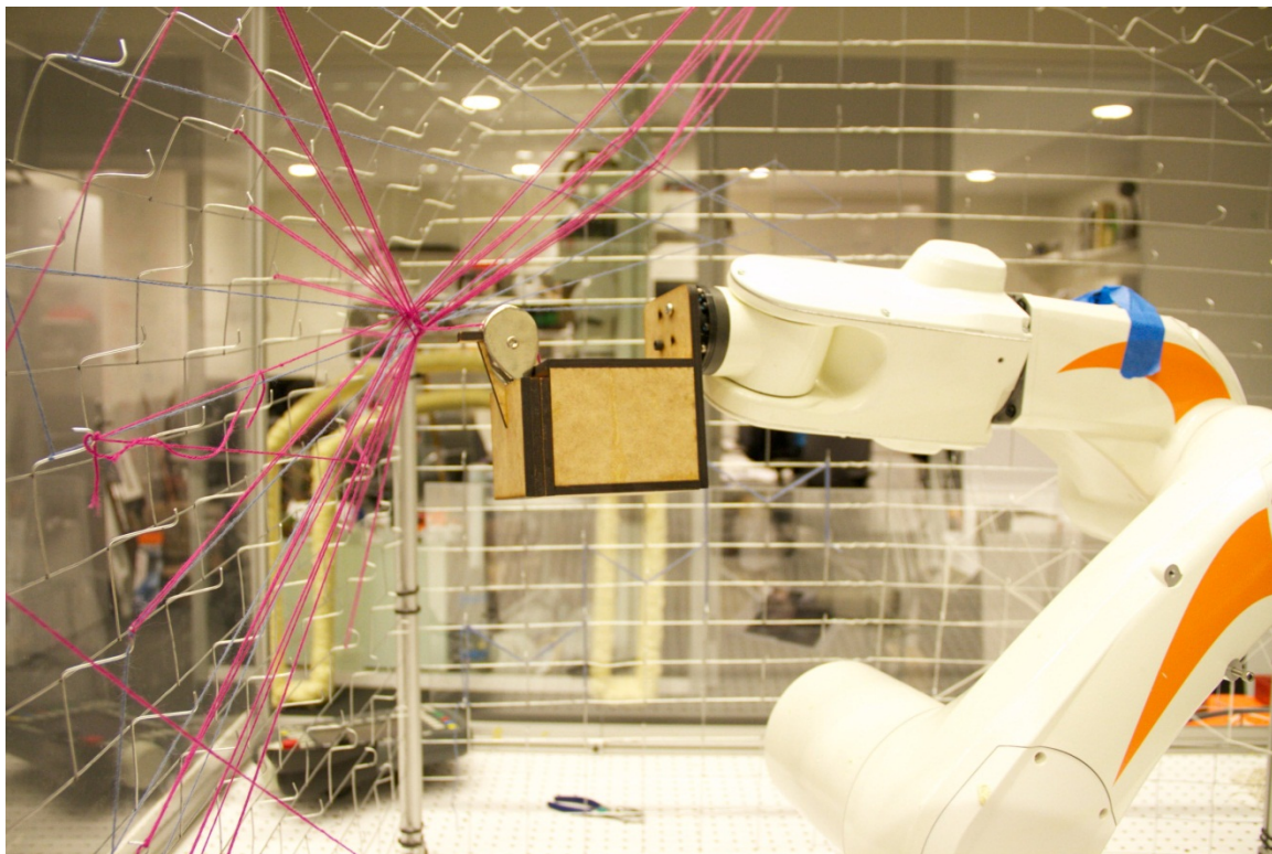
Figure 2 Image of the KUKA arm with a holder attachment containing a spool of yarn. The arm is inside a metal frame enclosure with protruding hooks serving as support for the yarn.
