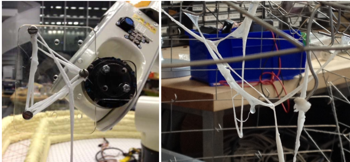
Figure 4 Robotic Arm manipulating the weaving frame that the nylon is being wrapped around. The nylon prepolymer solution is resting on the table below the arm (left). Nylon threads attached to hooks on a steel frame formed by dipping the hooks into a nylon prepolymer solution.
