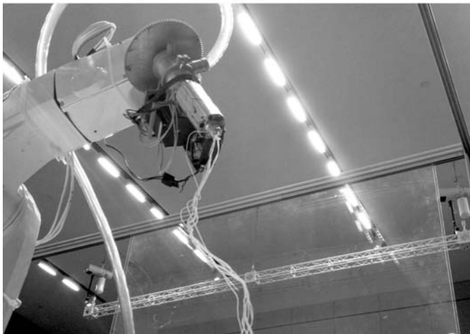
Figure 4. SEM image of silk fibers (top left), HDPE extrusion (top right), and thermoplastic extruder on KUKA robotic arm (bottom).
