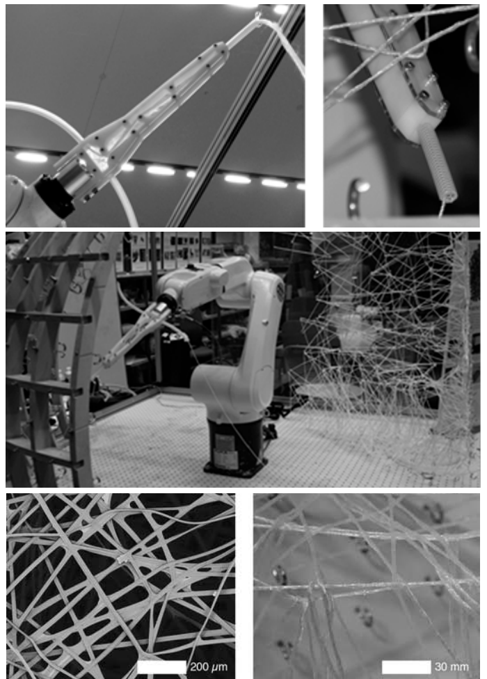
Figure 5. Fiber pulling tool (top), fiber pulling tool on KUKA robotic arm with external hook structure (middle), comparison of epoxy resin-soaked polypropylene twine (bottom right) and SEM image of scaffolding silk fiber (bottom left).
