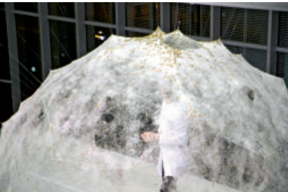
Fig. 13: Top view of the Silk Pavilion as approximately 6500 silkworms construct the fibrous composite.
