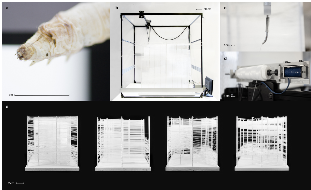
Figure 1: Construction setup and tools. (a) Bombyx mori silkworm. (b) Custom gantry with woven structure scale model (1:5) inside. (c) Fiber deposition nozzle. (d) Solenoid tensioning mechanism. (e) 1:33 scale models.
