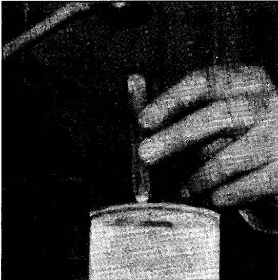
Applying Mold Marking with Stamp
