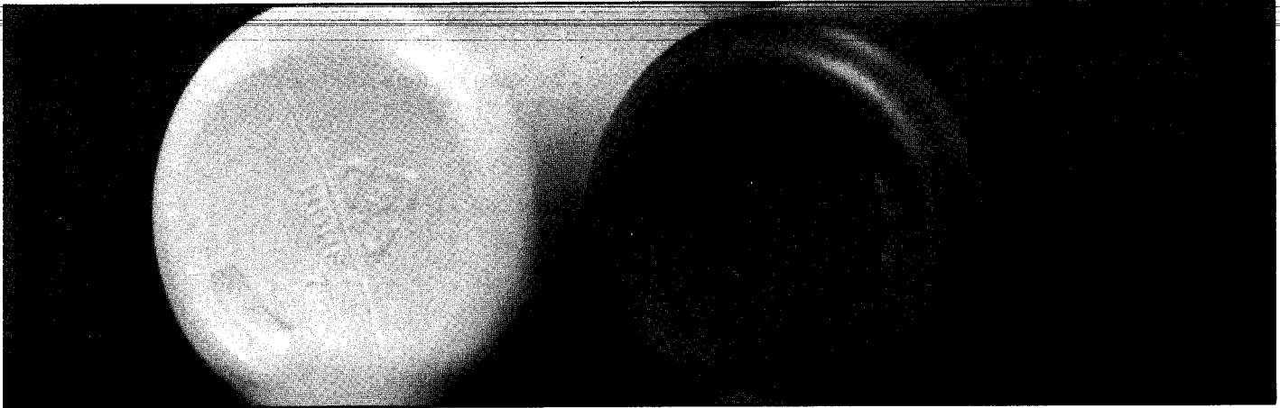
Finished Bottles with Molded Code
