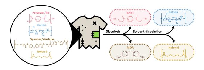
Overview of the chemical full recycling process. Conversion of real mixed textile waste (polyester, cotton, spandex, and nylon) using MW-assisted glycolysis and solvent dissolution. BHET, bis(2-hydroxyethyl) terephthalate; MDA, 4,4'-methylenedianiline. Credit: *Science Advances* (2024). DOI: 10.1126/sciady.ado6827
