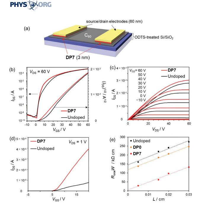
a) Schematic device structure, b) transfer curves in the saturation regime, c) output curves, d) transfer curves in the linear regime of  $C_{60}$  undoped (black) and contact-doped with DP7 (red) OFETs with *W/L*. Credit: *Advanced Materials* (2024). DOI: 10.1002/adma.202311047
