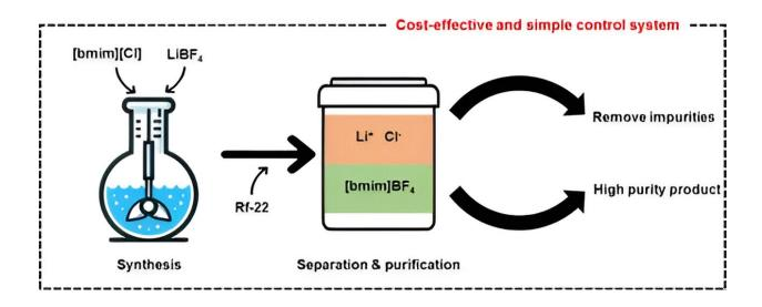
Schematic of ionic liquid synthesis and purification process. Credit: *Industrial & Engineering Chemistry Research* (2024). DOI: 10.1021/acs.iecr.4c01218
