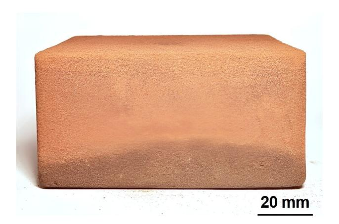
Photograph and X-ray CT image of KLS-1 sintered block manufactured using an optimized process. Credit: Korea Institute of Civil Engineering and Building Technology
