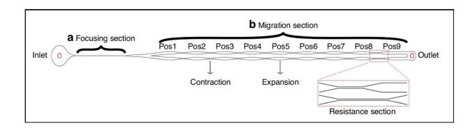
A schematic of the design of the microfluidic chip. The inlet is followed by a
