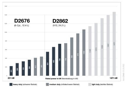
MAN Engines covers a broad power portfolio from 221 to 1471 kW in the IMO Tier III emission level.
