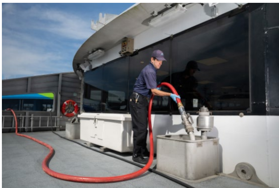
Refueling a ferry with HVO
