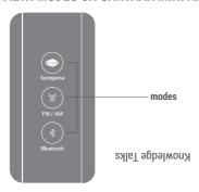
To choose a mode, press the corresponding mode button on the unit
