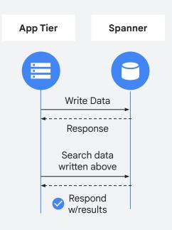
The diagram below conveys the potential for search queries against recently written data in traditional OLTP + Search architecture returning stale results due to the data copy lag associated with the ETL process. With Spanner FTS on the other hand, you always get real-time, transactionally-consistent search results.
