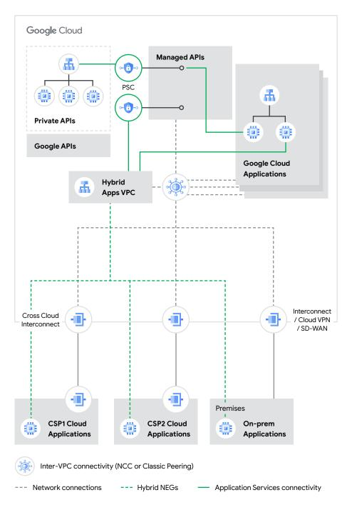
The PSC and load balancing components of the service centric network also enable the insertion of service extensions that enable the seamless integration of routing, security and traffic functionality across the application stack. Service extensions make the Cross-Cloud Network extensible and open by enabling the seamless integration of an open ecosystem of partner solutions.
