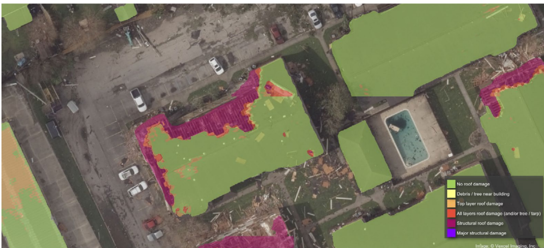
Figure 2: Output of damage segmentation model developed and used by Munich Re.
