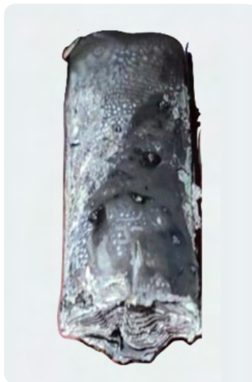
Third-party battery after an External Short-Circuit test, which is intended to simulate an unintended circuit fault.
