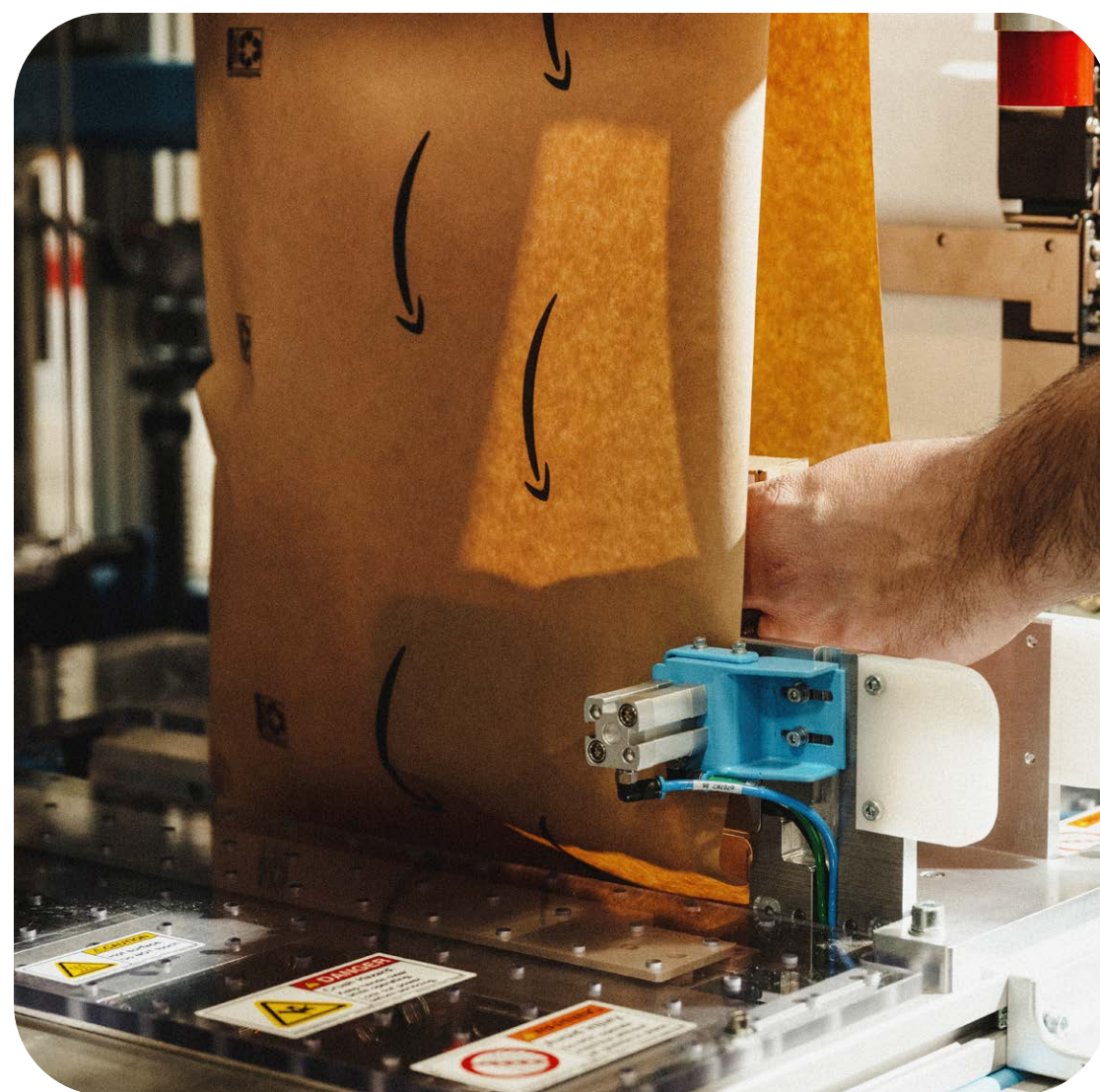
We’re testing new packaging machines in Europe and the U.S. that build made-to-fit paper bags around individual items on demand.
