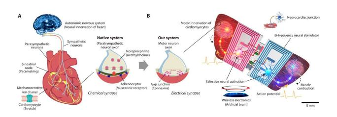
Wirelessly controllable bioelectronic neuromuscular robots for steering actuation behavior. (A) Dynamic control of the heart via the neural innervation of cardiomyocytes (CMs). (B) Schematic of a bioelectronic neuromuscular robot with selective motor innervation of CMs driven by a wireless frequency multiplexing bioelectronic device. Credit: Hiroyuki Tetsuka
