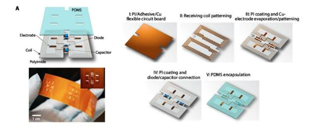
Fabrication process for the flexible PCB-based wireless bi-frequency bioelectronic device. Credit: Hiroyuki Tetsuka
