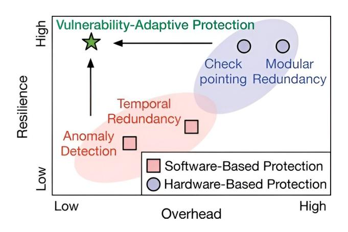
Design landscape of different software and hardware-based protection techniques for resilient autonomous machines. Our proposed vulnerability-adaptive protection design paradigm co-optimizes performance, energy efficiency, and resilience. Credit: *Communications of the ACM* (2024). DOI: 10.1145/3647638
