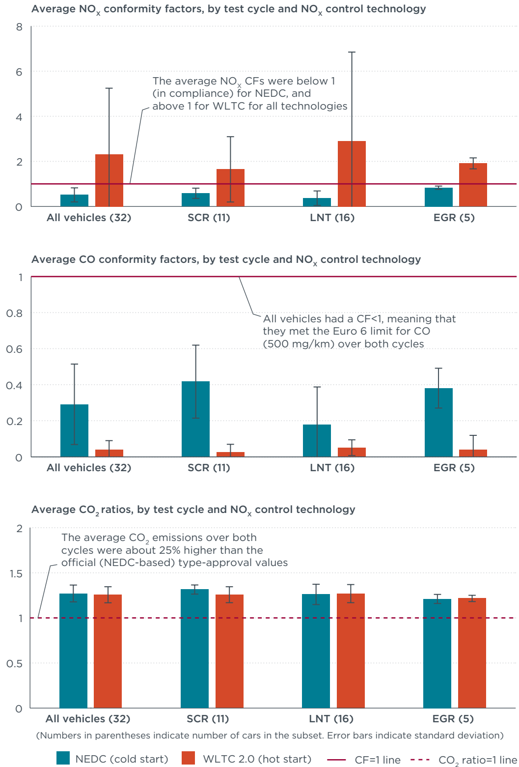
Figure 7: Average experimental conformity factors for NO x and CO, and CO 2 ratios, by test cycle and NO x control technology
