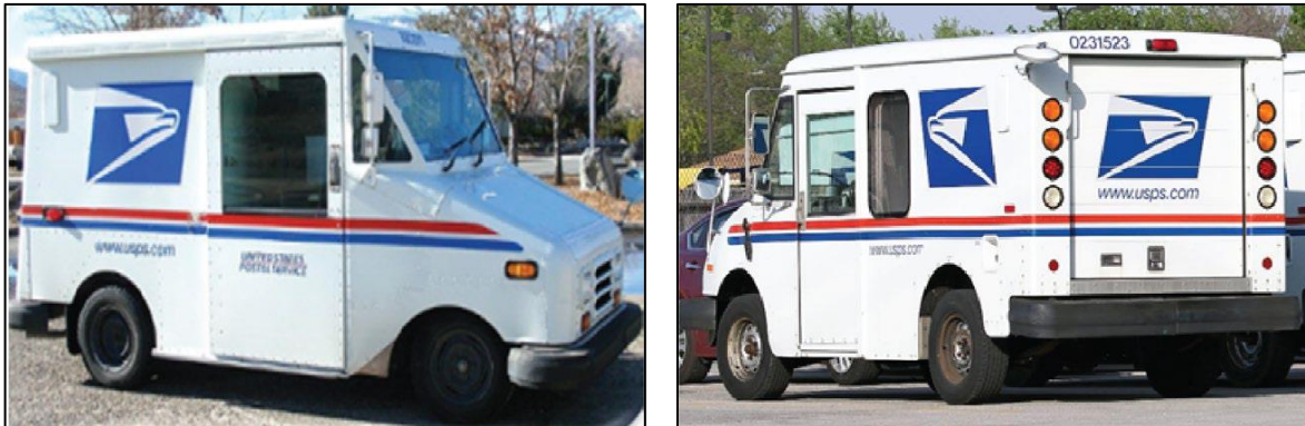
Figure 2-1.1 Example of RHD LLV (on left) and RHD FFV (on right) (OIG 2020)
