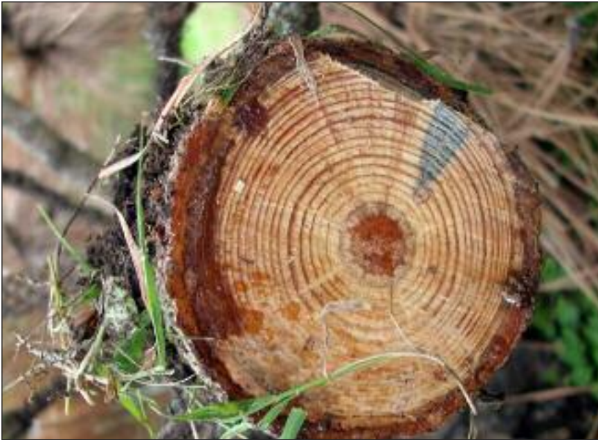
Blue staining of timber symptomatic of Diplodia spp. infections (RBG Melbourne)
