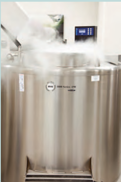
An open liquid nitrogen tank at the Smithsonian's Biorepository. (Donald E. Hurlbert)
