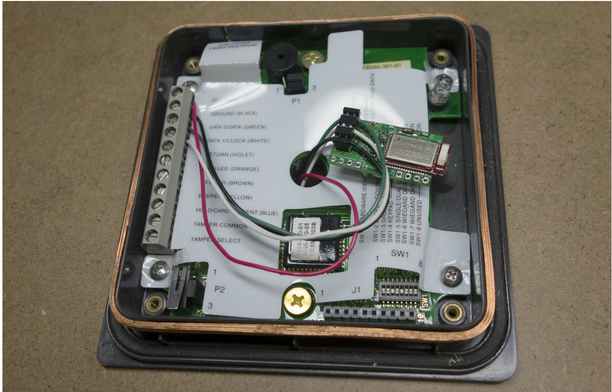
Figure 4: BLEKey installed in a popular RFID reader.
