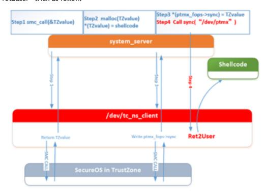
I choose TEE OS's internal time as a given returned value. The global service in TEE provide a time query interface with cmd\_id = "GLOBAL\_CMD\_ID\_TEE\_TIME".
