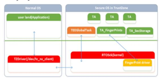
TZDriver "/dev/tc\_ns\_client" is a kernel driver which provides an interface to user space clients for communication with TEE OS. Just like "/dev/qseecom" in QSEE.The only diffirent is every local Android application can access TZDriver on mate 7, qseecom only can be accessed by some system process.
