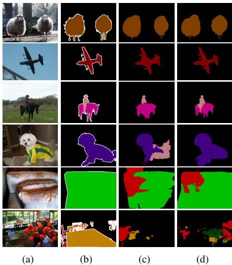
Figure 4: Qualitative segmentation results on PASCAL VOC 2012 val set. (a)-origin image, (b)-ground truth, (c)-results of Song et al. [23], (d)-ours.
