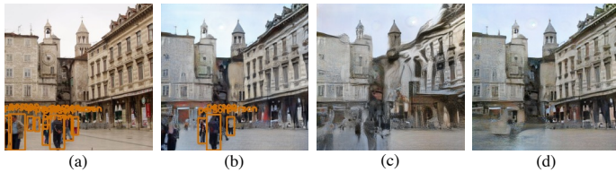
Figure 1: Reverse Engineering Attack and Mitigations. (a) Original image. Objects detected marked in orange (b) Reverse-engineered image using our attack. The reconstruction preserves semantic information. By (c) reducing the number of features or (d) selective suppression around private objects, we reduce the efficacy of the attack and improve privacy.
