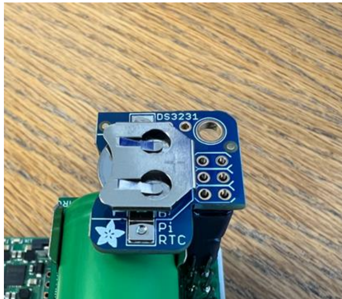
Figure 11: Image of RTC installed on the raspberry pi and super watchdog
